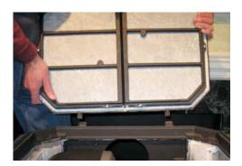
3. Using a 1/2" wrench or socket, remove the two bolts annu washers that hold the combustor cells and combustor frame (W-165/166) in place. (These bolts do not need to be reinstalled as they are for transport only).
