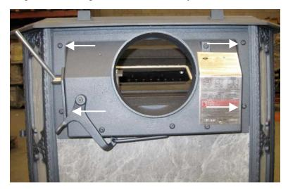
**8.** Reach into the firebox and remove the combustor scoop (W-249) and metal diffuser (W-305) by removing the single bolt that attaches it to the combustor pan scoop support (1/2"wrench or socket to loosen). Carefully slide the scoop toward the loading door and forward to completely release it. **Be very careful with the metal diffuser it is extremely sharp around the edges.**
