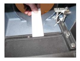
28. Apply cement in the gap around the top edge of the air duct cover and carefully place 1/4" gasket around the channel. Use 3/16" gasket in areas where the gap is too small for 1/4". If you press to hard the gasket will go through into the stove. Repaint if desired.
