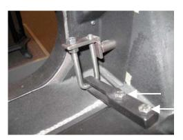
5. Using the large flat blade screwdriver, remove the four bolts that hold the top half of the combustor assembly (air duct cover, W-163). Make a note of their positions as all the screws are not the same length. Lift the cover up and off the assembly.
