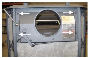
27. Attach the bypass lift guide to the bypass door using 1" stainless steel bolts and a 1/2" wrench or socket. Adjust for proper tension on the bypass door so it has a seal with the gasket underneath it. Slide a small piece of paper under it, close the bypass door, and pull the paper out. There should be resistance and the paper should curl up.
