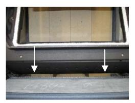
17. Run a bead of cement between the two spacers and the comb. pan, and then smooth out the cement with your finger to ensure cement gets pressed into the seams. (The size of the combustor pan varies a little. If need be, push a piece of gasket between the combustor pan and the spacer before cementing.)
