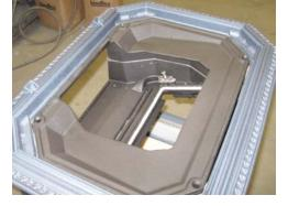
24. Install the four flat head screws into the air duct cover as follows: 2" in the right front, 4" in the left rear, and 5" into the last two, tighten.
